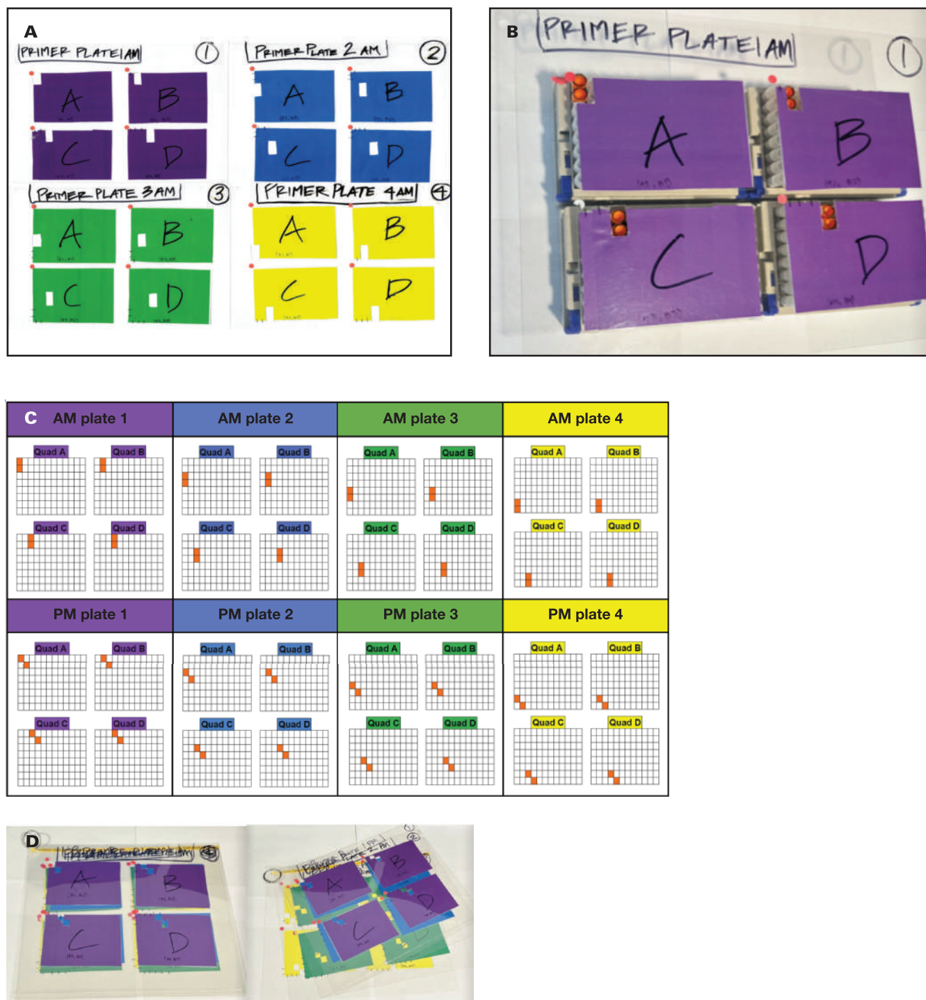
FIGURE 1. A, Two-dimensional printed templates for the AM run with 4 primer plates. Holes in the templates correspond to the correct placement of the control tubes when the template is placed on top of specimen racks and the colors represent the 4 primer plates. B, The 2D template for primer plate 1 of the AM run in use on top of 4 specimen racks indicating the placement of control tubes (orange caps). C, Schematics for control tube placements for each of the 4 primer plates for AM and PM runs. Each color represents a plate number whereas the orange squares represent correct control tube placements. D, Two-dimensional templates for AM and PM runs for the 4 original primer plates. Each laminated sheet represents a 384 well plate consisting of 4 racks of 96 patient sample tubes and the templates for each of the 4 primer plates are bound with a metal ring.
