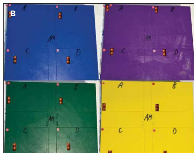
FIGURE 2. A, CADD file showing the design of our 3D templates designed to fit on top of 4 specimen racks. Importantly, the “G” dimension ensures that the template remains on top of the set of tubes without sliding. B, AM run 3D templates are shown on top of specimen racks with orange specimen tube caps representing the control tubes. The color of the template corresponds to the respective primer plate number 1-4.
