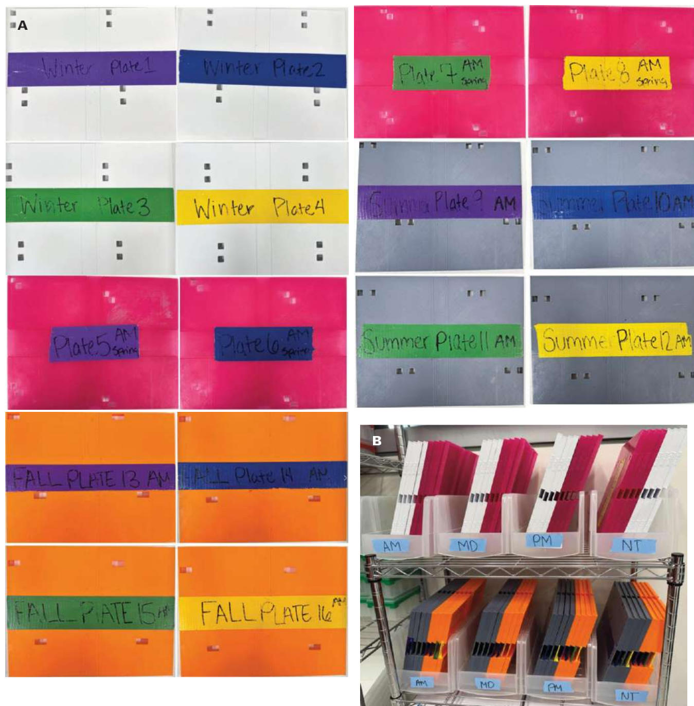
FIGURE 4. A, Current set of 3D printed templates for midday (MD) run configuration. The template colors (white, pink, orange, and gray) represent each of the 4 seasonal groupings whereas the tape color represents each of the 4 primer plates within that season. B, Shelves and bins containing all 16 3D printed templates organized for each season set. Each color of the 3D printed template represents the set of 4 plates for its respective season. Each 16-set of templates has unique control tube placements for MD, PM, and nighttime (NT) runs. This organizational system allows operating technicians to quickly and simply identify the proper templates for the run they are performing.
