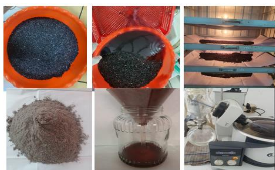
Figure 1. Process for Making Black Rice Extract
