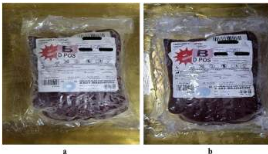
Figure 4 Film indicator before (a) and after (b) irradiation (25 Gy).
