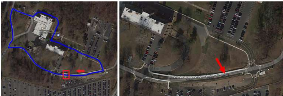
Fig. 4. (Left to right) Test track with direction and crosswalk location, distance from crosswalk where message is to be sent to the driver.
