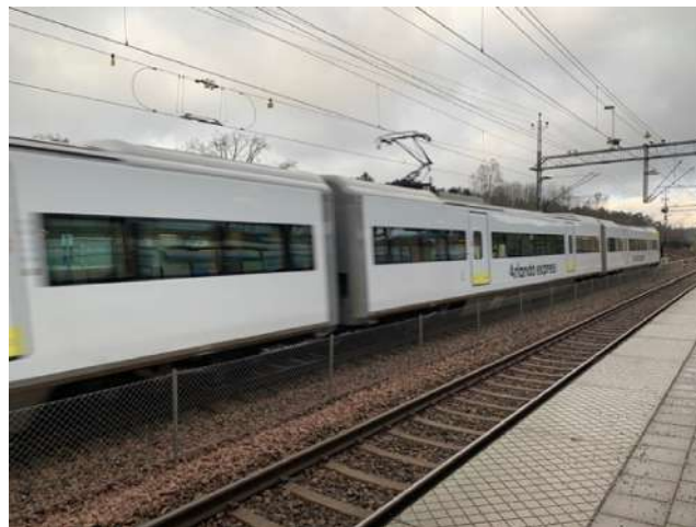
Fig. 1. Photo of the installed mid-track fence and a high-speed train passing by the intervened station. The lower speed commuter train track which has trains stopping at the station, is to the right of the high-speed train track in the picture. Also refer to the Supplement for a brief discussion about the fence design.
