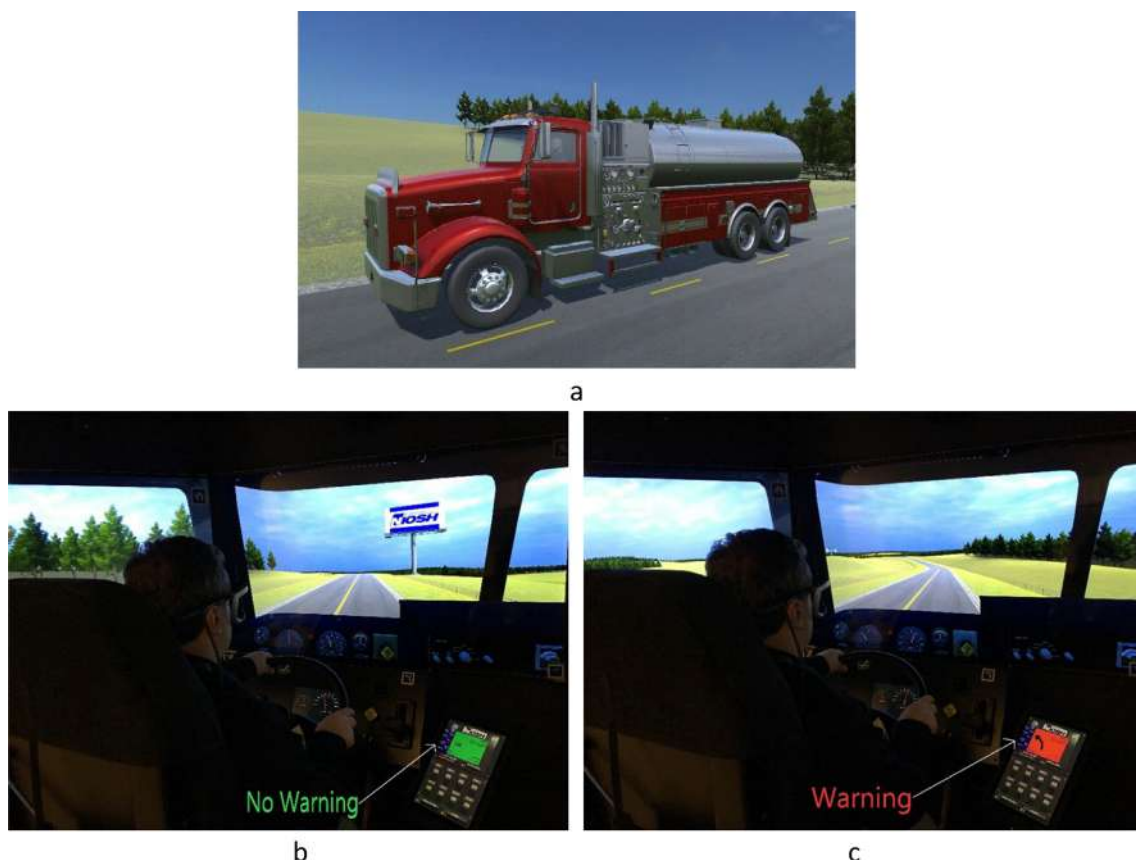
Fig. 1. Selected simulations: (a) fire tanker model; (b) view from the cab, with active CSWS while driving on a straight section within the safety speed limits (green screen); (c) approaching a curve with inappropriate speed – the active CSWS is issuing a warning (red screen).
