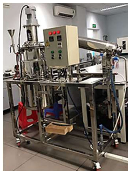
Fig 1. Hydrodistillation equipment 50 L/batch
