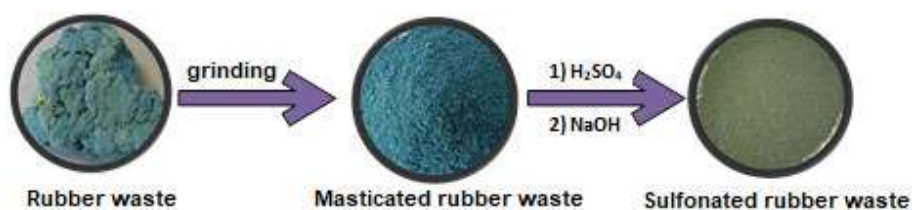
Fig 1. The sulfonation reaction of the rubber waste
