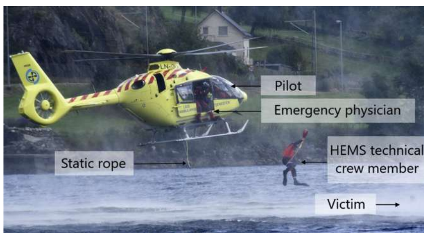
Figure 1. Ihopp: the primary static rope over water procedure in Norwegian HEMS (courtesy of Fred Sirevaag).
