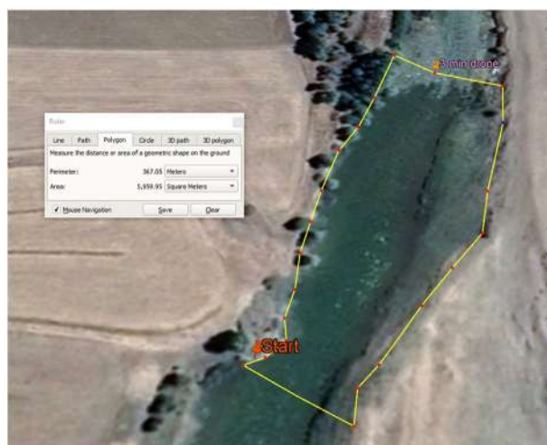
Figure 5. Method of calculating the area of the riverbed scanned from the starting point to the point of first visual contact (using Google Earth Pro).
