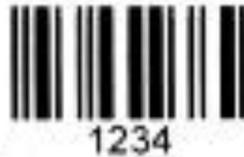
Gambar 2.3 *Barcode* Jenis Interleaved 2 of 5
