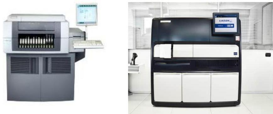
**Gambar 2.5** Alat uji saring metode ChLIA (Architect i1000 System dan Diasorin Liaison XL Analyzer) (wegomedika.com & labx.com)
